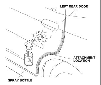
12. Open the left rear door again. Peel back about 50 mm (2 in.) of adhesive backing from the left rear door edge film. Align the V-notch in the door edge film with the end of the character line on the upper part of the left rear door.
