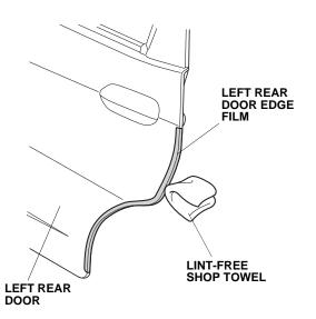
18. Repeat steps 10 through 17 to install the door edge film on the right rear door.
