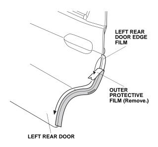
16. Starting in the middle of the door edge film and working outward, fold the film around the door edge using your fingers. Move your fingers in one direction. Attach the film over the seam sealant. Do not trim or damage the seam sealant.
