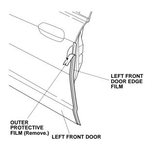
7. Starting in the middle of the door edge film and working outward, fold the left front door edge film around the door edge using your fingers. Move your fingers in one direction. Attach the film over the seam sealant. Do not trim or damage the seam sealant.
