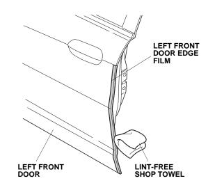
9. Repeat steps 1 through 8 to install the door edge film on the right front door.
