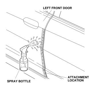
3. Open the left front door again. Peel back about 50 mm (2 in.) of adhesive backing from the left front door edge film. Align the V-notch in the door edge film with the end of the character line on the upper part of the front door.
