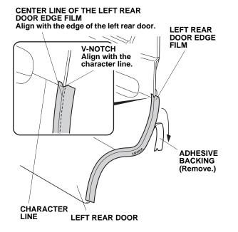
13. Continue to remove the adhesive backing while you align the center line on the door edge film with the edge of the door.
