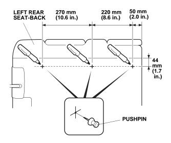
4. Insert the snaps through the covers, then install the snaps at the pierced marks.
