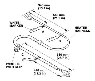
11. Plug the connector of the heater harness into the engine block heater, and route the heater harness over the engine. Secure the heater harness to the vehicle harness with one white wire tie in the area shown.
