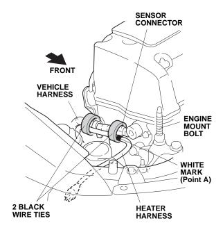
14. Continue routing the heater harness under the ABS unit bracket along the vehicle harness, and secure the heater harness to the vehicle harness with two black wire ties in the areas shown.
