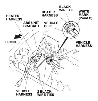
15. Route the heater harness as shown, then secure the harness with two black wire ties in the areas shown.
