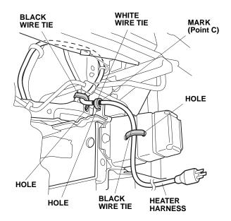
19. Route the heater harness as shown. Reinstall the front bumper in the original position.
