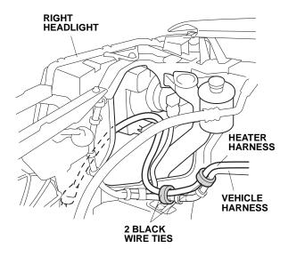
Route the heater harness as shown. Attach the wire tie with clip to the vehicle panel hole.
