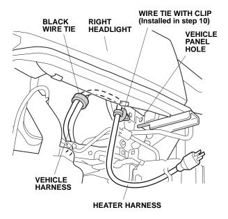
17. Using one black wire tie, secure the heater harness to the vehicle harness.
