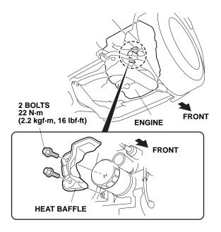
7. From the underside of the vehicle, remove the two bolts and remove the heat baffle from the engine.
