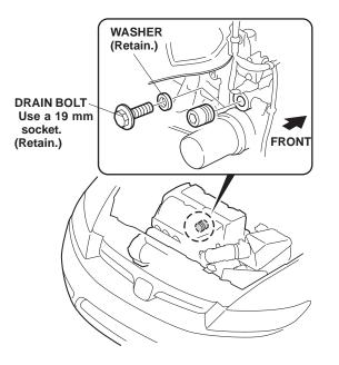
Install the new aluminum washer and the engine block heater into the bolt hole using a 24 mm socket and a torque wrench. Torque the engine block heater to 60 N·m (44 lb-ft).
