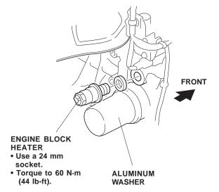
16. Route the heater harness down to the engine block heater. Connect the heater harness connector to the engine block heater.
