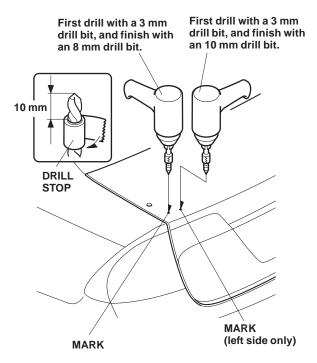
12. Open the trunk lid. Route the harness on the trunk spoiler down through the 10 mm hole you just drilled. Attach the grommet on the trunk spoiler harness to the 10 mm hole.
