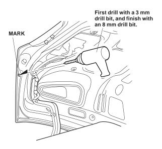
7. Mark the trunk lid stop with a felt-tip pen, then turn it counterclockwise to remove it. Repeat on the other side.
