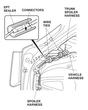
34. Make loops in the trunk spoiler harness, then secure the trunk spoiler harness and spoiler harness to the vehicle harness with two wire ties as shown.
