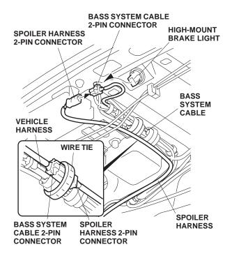
26. Gently pull down the right trunk panel, and locate the clip on the vehicle harness attached to the rear shelf. Align the green tape on the spoiler harness with the clip on the vehicle harness, and secure the spoiler harness to the vehicle harness with one wire tie in that area.
