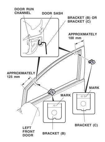
19. Hook the front bracket on the left front door visor on the door sash, and install it so that there is no space between the bracket and the door sash.
