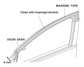
27. Peel back 1½ to 2 inches of adhesive backing from each adhesive tape, and tape the ends to the front surface of the door visor with masking tape..
