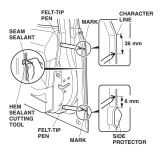
9. Position the hem sealant cutting tool against the door edge, and trim the seam sealant from mark to mark.
