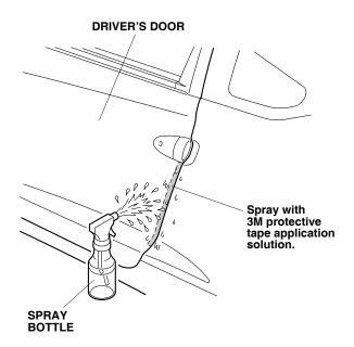
Open the driver's door. Peel back about 50 mm of the adhesive backing from the left door edge film. Align the v-notch on the left door edge film to driver's door as shown.
