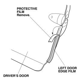
7. Starting from the top and working downward, use the applicator and soft sleeve to fold the left door edge film inside the driver's door as shown.
