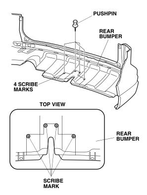
26. While wearing an eye protection, drill the rear bumper at each pierced mark using a 20 mm hole saw.
