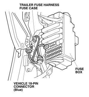
53. Secure the trailer fuse harness to the vehicle harness with two wire ties.
