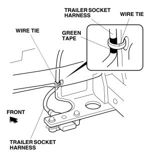
34. Using isopropyl alcohol on a shop towel, thoroughly clean the two areas where the harness tapes will attach. Attach one harness tape to the edge of the vehicle panel, and attach the other harness tape to the vehicle panel to secure the trailer socket harness.
