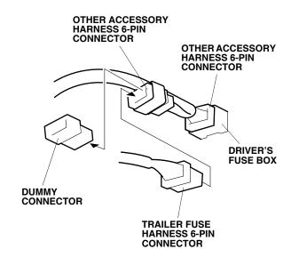
52. Secure the fuse case on the trailer fuse harness to the vehicle 18-pin connector (blue).
