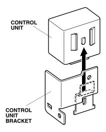
41. Plug the control unit harness 12-pin connector into the control unit, then secure the control unit harness to the control unit bracket using the wire tie with clip installed in step 39.
