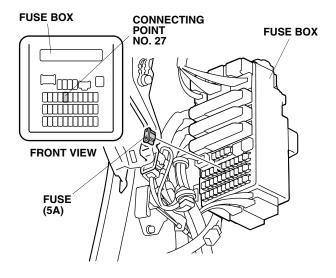
55. If an optional 5A fuse label is already attached to the driver's dashboard under cover, go to step 56. Otherwise, using isopropyl alcohol on a shop towel, thoroughly clean the area where the fuse label will attach. Attach the 5A fuse label to the NO. 27 slot on the driver's dsshboard undercover.
