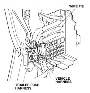
54. Insert the 5A fuse into the fuse box at the empty slot shown.
