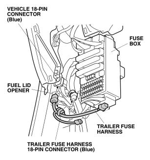
50. Plug the trailer fuse harness 6-pin connector to the 6-pin opening in the fuse box.
