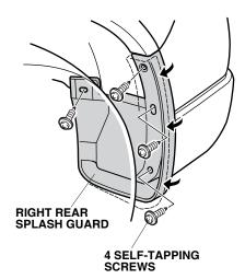
4. Remove the right rear splash guard (four screws and slide forward).
