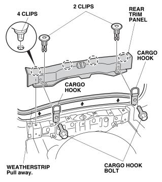
14. Pull away the tailgate weatherstrip, and remove the rear trim panel (four clips and two clips).
