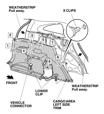
17. Remove the left cargo area side trim panel by releasing the eight clips in the order shown, and unplugging the vehicle connector.
