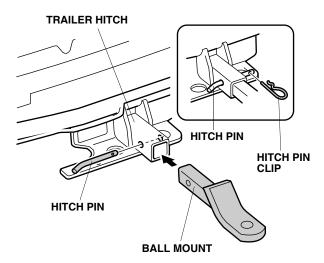
After the first 600 miles (1,000 km) of towing, have your Honda Dealer recheck the torque of the trailer hitch bolts.
