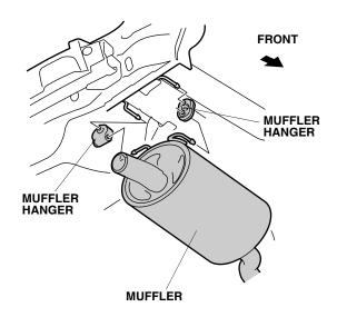
20. Install the two muffler hangers (removed in step 19) onto the hooks of the trailer hitch at the locations shown.
