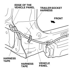
35. Inside the vehicle along the cargo area left panel, locate the vehicle 8-pin connector blue-taped to the vehicle harness. Remove the blue tape to free the connector.
