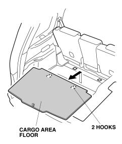
13. Remove the cargo hooks (one bolt for each hook).
