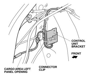
45. Loosely thread the 6 x 16 mm flange bolt into the control unit bracket.
