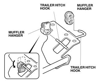
21. With the help of an assistant, install the trailer hitch on the vehicle using the six 10 x 40 mm hex bolts with spring washers and plain washers. Do not tighten the bolts at this time.
