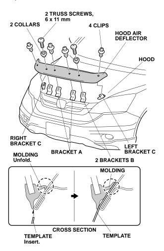
17. Using the large end of a template, insert it between the hood and hood air deflector to unfold the molding as shown.
