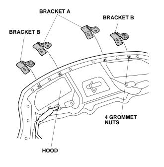
3. Close the hood. Attach pieces of masking tape to the hood under two brackets A and two brackets B as shown.
