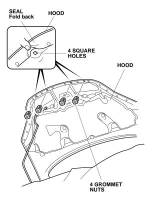
2. Align two brackets A and two brackets B to the holes on the four grommet nuts.
