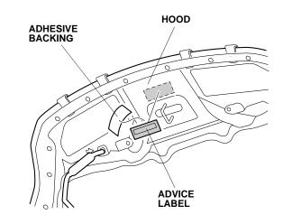
19. Remove the adhesive backing from the advice label and attach it to the hood as shown.
