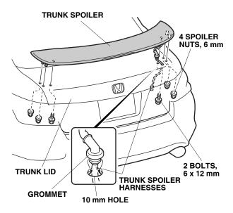
13. Fit the trunk spoiler into position on the trunk lid, and install the four 6 mm spoiler nuts and two 6 x 12 mm bolts. Hold the trunk spoiler firmly against the trunk lid and torque the spoiler nuts and bolts to 9 N·m (6.5 lb-ft).
