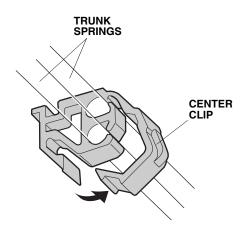
17. With an assistant holding the trunk lid open, use the trunk spring tool to remove the old trunk springs from the trunk hinge arms. Wear gloves to protect your hands, and pull the trunk spring tool slowly and carefully towards you.
