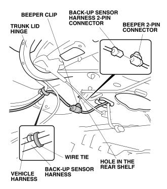
26. Secure the back-up sensor harness to the vehicle harness using one wire tie.
