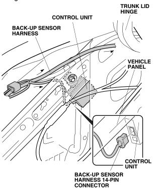
Secure the back-up harness to the vehicle harness with two wire ties.
