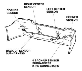
36. Install the two clips on the back-up sensor subharness into the holes in the left center sensor clip and the right center sensor clip.
