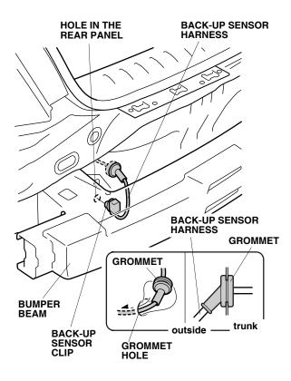
30. Attach the clip on the 8-pin connector into the hole in the rear panel.
