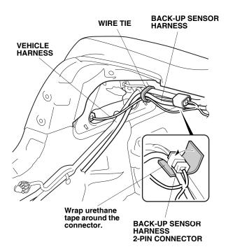
15. Plug the back-up sensor harness 14-pin connector into the control unit, and route the harness forward along the vehicle harness.
