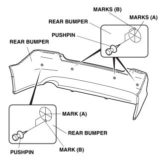
32. While wearing eye protection, drill all eight pierced marks using a 3 mm drill bit.
