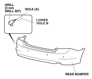
Using a 24 mm hole saw, enlarge the outboard (right and left corner sensor) bumper holes. On the driver's side, drill the LOWER 3 mm hole. On the passenger's side, drill the UPPER 3 mm hole.
