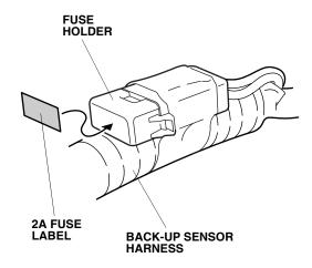
13. Disconnect the back-up light 2-pin connector from the left taillight, and plug it into the back-up sensor harness 2-pin connector. Plug the remaining back-up sensor harness 2-pin connector into the left taillight.
