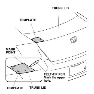
7. Flip the template over. Align the template with the right side trunk lid. Using a felt-tip pen, make two marks on the right side trunk lid as shown. Remove the template.
