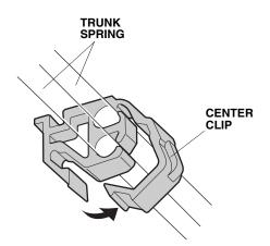
18. With an assistant holding the trunk lid open, remove the old trunk springs from the trunk hinge arms using the trunk spring tool. Wear gloves to protect your hands, and pull the trunk spring tool slowly and carefully toward you.
