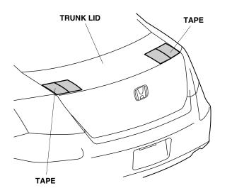
6. Align the template with the left side trunk lid. Using a felt-tip pen, mark the left side trunk lid as shown. Remove the template.
