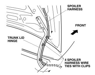
33. Route the spoiler harness and secure the two spoiler harness wire ties with clips to the vehicle panel holes.
