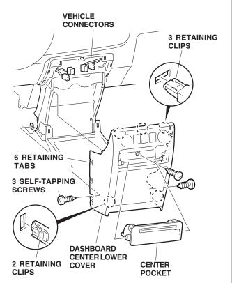
6. Insert a flat-tip screwdriver with a shop towel wrapped around it into the groove of the instrument panel, and release the clips. Pull the instrument panel out toward you to release the eighteen clips, and unplug the vehicle connectors. Remove the instrument panel.
