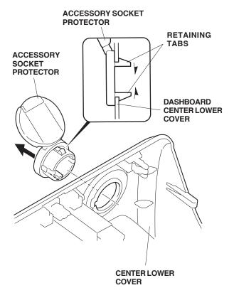
Slide the lighter ring into the hole in the front dashboard center lower cover in the direction shown.
