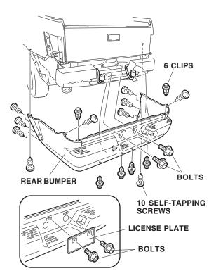
26. On the inside of the rear bumper, locate the six marks. Center punch the six marked locations on the rear bumper. While wearing eye protection, drill a 1 3/16 in. (30 mm) hole through each marked location. First drill with a 3 mm drill bit, and then finish with a 1 3/16 in. (30 mm) holesaw. Remove all burrs from the edges of the holes with a file.
