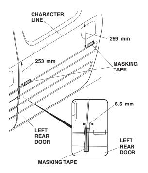
On the inside of the left rear upper molding, attach a strip of masking tape to the ends of the long adhesive backing and peel back 1-1/2 to 2 in. (3-5 cm) from the adhesive backing. Tape the ends to the front of the moldings. Remove and discard all other adhesive backings.
