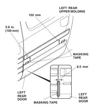
On the inside of the left rear lower molding, attach a strip of masking tape to the ends of the long adhesive backing and peel back 1-1/2 to 2 in. (3-5 cm) from the adhesive backing. Tape the ends to the front of the moldings. Remove and discard all other adhesive backings.
