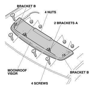
Adjust the position of the moonroof visor. Check that the brackets A and brackets B are firmly secured. Make sure the rubber molding on the moonroof visor is not twisted or rolled under the visor.
