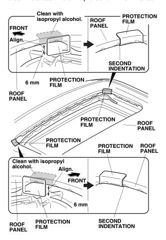
4. Remove the adhesive backings from the protection film. Starting from the bottom edge of the protection film, wrap 6 mm of the protection film around the lip of the roof panel opening and align it with the second indentation on the left side of the roof panel as shown; continue upward with the protection film around the top of the roof panel. Repeat the procedure on the right side of the roof panel.
