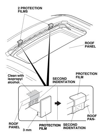
6. Remove the adhesive backings from the protection film. Starting from the bottom edge of the protection film, wrap 3 mm of the protection film around the lip of the roof panel opening to cover the second indentation on the left side of the roof panel; continue upward with the protection film around the top of the roof panel. Repeat the procedure on the right side of the roof panel.
