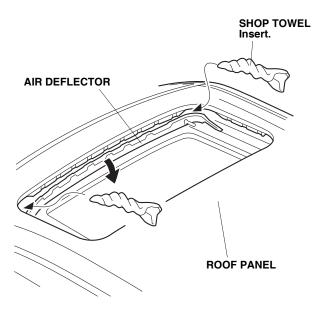
2. Roll up two shop towels and insert them between the roof panel and air deflector to lower the air deflector. Do not to damage the air deflector.
