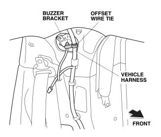
27. Route the buzzer harness along the vehicle harness, and secure it to the vehicle harness with two wire ties.
