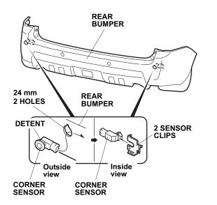
55. Install the two center sensors on the rear bumper using one sensor clip for each sensor.
