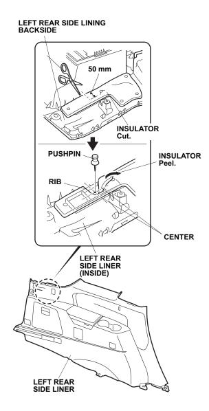
44. Using a pushpin, mark the left rear side liner in the center of the square as shown.
