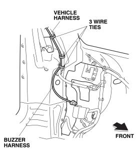
29. Plug the buzzer connector to the control unit. Bundle up the excess buzzer harness and loosely secure it to the vehicle harness with one wire tie.
