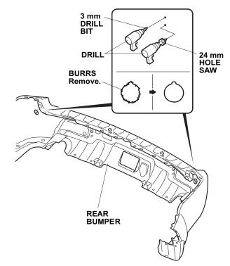
53. While wearing eye protection drill the right center mark at the upper pierced mark with a 3 mm drill bit. On the left center mark, drill the lower pierced mark with a 3 mm drill bit. Then drill the two center marks using a 26 mm hole saw. Remove all burrs.
