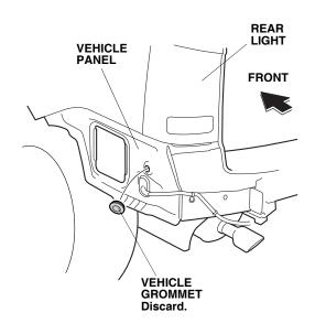
40. Route the back-up sensor harness through the vehicle grommet hole, and install the back-up sensor harness grommet onto the vehicle panel.
