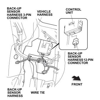
33. Route the back-up sensor harness 3-pin connector as shown and secure it to the vehicle harness with two wire ties loosely secured in step 29 and 30.
