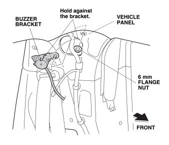
26. Secure the vehicle harness to the buzzer bracket with the offset wire tie as shown.
