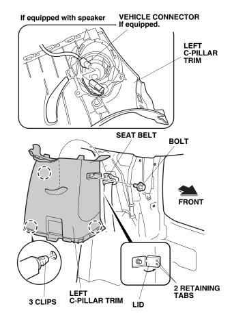
16. Using a small rubber mallet and a shop towel, gently tap the left C-pillar trim at the area marked "SIDE CURTAIN AIRBAG" to release the clip.
