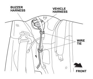
28. Secure the buzzer harness to the vehicle harness with three wire ties.
