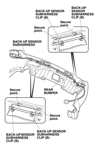
59. Using an isopropyl alcohol on a shop towel, clean the area where the harness tape will attach. Secure the back-up sensor subharness to the rear bumper with one harness tape.
