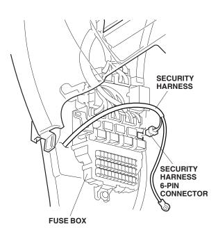
NOTE: If another accessory is already plugged into the 6-pin connector, remove the dummy connector from the other accessory harness and plug the security harness into that connector.
