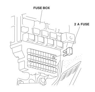
27. Attach the 2 A fuse label to the No. 33 slot on the fuse box cover.
