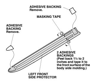
5. Align the left front body side molding with the front template, and attach it to the left front door. If the vehicle has door edge film installed, align the end with the door edge film.
