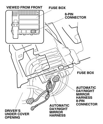
• If the fog light connector is already plugged to the fuse box 8-pin connector, remove the dummy connector from the automatic day/night mirror harness. Unplug the fog light 8-pin connector, and plug it into the automatic day/night mirror harness. Plug the automatic day/night mirror harness 8-pin connector into the fuse box 8-pin connector.
