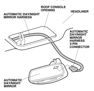
24. Route the automatic day/night mirror harness through the groove on the harness cover. Secure the harness cover to the stay, and slide the harness cover under the headliner.
