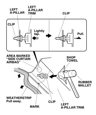
10. Using a rubber mallet wrapped with a shop towel, lightly tap the right A-pillar trim where it says "SIDE CURTAIN AIRBAG" to release the clip. 11. Pull away the rest of the weatherstrip and remove the right A-pillar trim (two clips).
