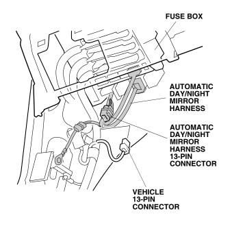
30. Remove and discard the upper bolt from the upper hood opener, and install the ground bolt supplied with the automatic day/night mirror harness ground terminal attached.
