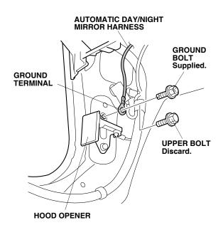
31. Secure the automatic day/night mirror harness to the vehicle harness with three wire ties.
