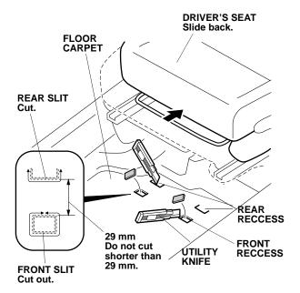
3. Locate the two front reccesses in the floor carpet. Using a utility knife, cut out each front reccess. Make sure the distance between the slit and the cutout is not less than 29 mm.
