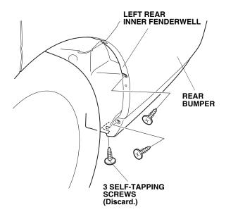
7. Secure the left rear splash guard with two 5 x 25 mm self-tapping screws and one 5 x 20 mm self-tapping screw, in the order shown.
