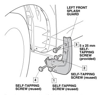
5. Turn the steering wheel fully clockwise and repeat steps 2 thru 4 to install the right front splash guard.
