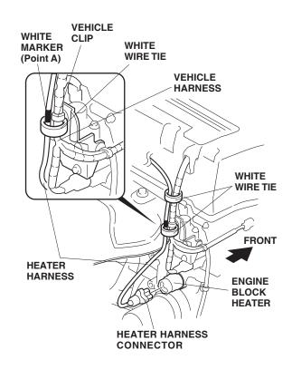
17. Secure the heater harness to the vehicle harness with one white wire tie at the marked point A. Then secure the heater harness to the vehicle harness, using another white wire tie above the marked point A. 18. Secure the heater harness to the vehicle harness with one black wire tie at the marked point B.
