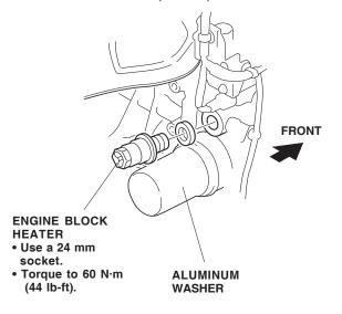
16. Route the heater harness down to the engine block heater. Connect the heater harness connector to the engine block heater.
