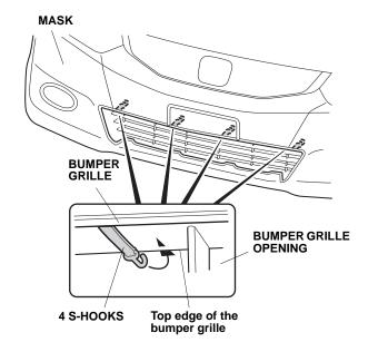
17. Attach the five S-hooks to the bottom inside edge of the bumper grille opening.
