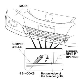
18. Attach the two hooks to the front bumper as shown.
