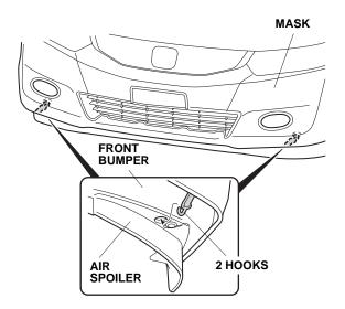
19. Route the elastic cord through the eight loops on the bottom of the mask. Attach one S-hook to the bottom edge of the bumper on one side. Stretch out the cord after routing it through each loop, then attach the other S-hook to the bottom edge of the bumper on the other side.
