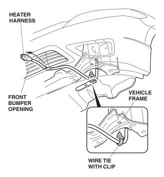
22. Secure the heater harness to the vehicle harness using five black wire ties.
