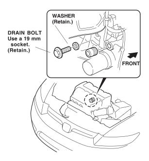
15. Install the new aluminum washer and the engine block heater into the bolt hole using a 24 mm socket and a torque wrench. Torque the engine block heater to 60 N·m (44 lb-ft).
