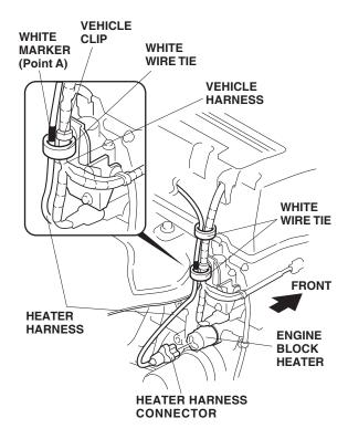
17. Secure the heater harness to the vehicle harness with one white wire tie at the marked point A. Then secure the heater harness to the vehicle harness, using another white wire tie above the marked point A.
