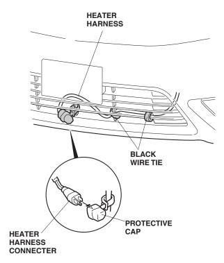
24. Attach the protective cap to the grille, and plug the heater harness connector into the protective cap.
