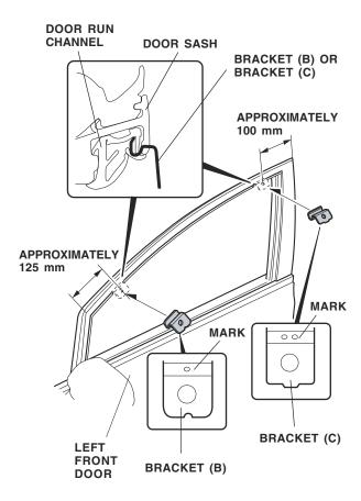
18. Install a bracket (B) and a bracket (C) on the door sash at the measurements shown. Verify the shape and the identification mark stamped on each bracket. Be sure to use the correct bracket at the proper location. 19. Hook the front bracket from the left front door visor on the door sash, and install it so that there is no space between the bracket and the door sash.
