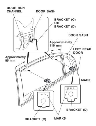
Install a bracket (C) and a bracket (D) on the door sash at the measurements shown. Verify the shape and the identification mark stamped on each bracket. Be sure to use the correct bracket at the proper location. 3. Position the left rear door visor on the door sash.
