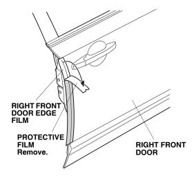
11. Starting from the middle and working outward, turn back the right front door edge film half to the cabin side of the right front door as shown. Move your fingers in one direction only.
