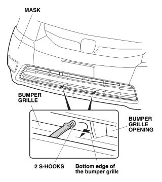
13. Route the elastic cord through the ten loops on the bottom of the mask. Attach one S-hook to the bottom edge of the bumper on one side. Stretch out the cord after routing it through each loop, then attach the other S-hook to the bottom edge of the bumper on the other side.
