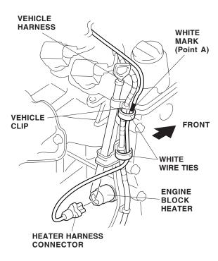
12. Secure the heater harness to the vehicle harness using two white wire ties. Attach one wire tie at the white mark (point A) made in step 8.
