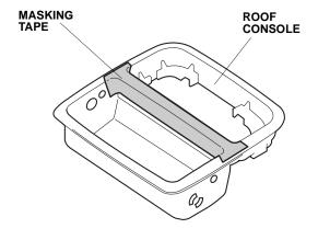
43. Attach template A to the roof console at the indicated position with masking tape.
