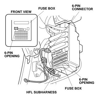
20. If another accessory is already plugged into the 6-pin connector, remove the dummy connector from the 6-pin connector taped to the HFL subharness. Plug the other accessory 6-pin connector into the HFL subharness and plug the HFL subharness into the fuse box. Repeat this step so that these accessories are connected in the following order: (HFL → Automatic Day/Night Mirror → Trailer Hitch).
