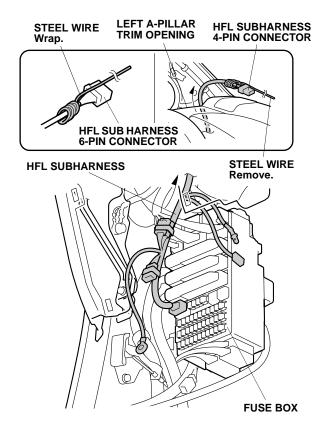
22. Remove the vehicle ground bolt. Place the HFL subharness ground terminal over the vehicle ground terminal, and secure them with the bolt.
