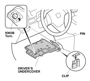
17. Remove the driver's dashboard lower cover (seven clips and two hooks). Be careful not to damage the clips and hooks.
