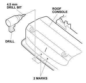
47. Using masking tape, attach the template B to the roof console at the indicated position.
