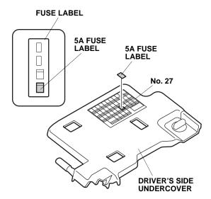
71. Attach the 5A fuse label to the Number 27 slot on the driver's undercover.
