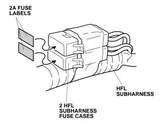
19. Plug the HFL subharness 6-pin connector into the 6-pin opening in the fuse box.
