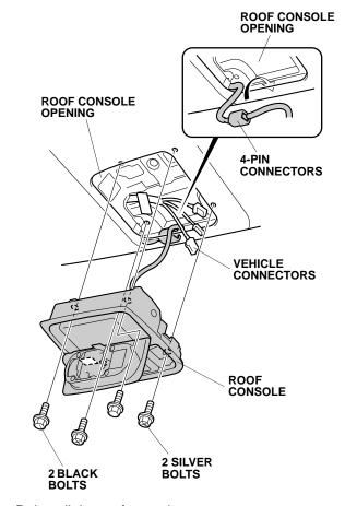
68. Reinstall the roof console.
