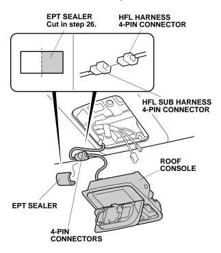
66. Wrap the piece of EPT sealer cut in step 26 around the 4-pin connectors.
