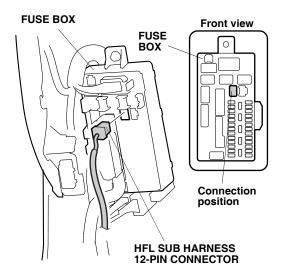
If another accessory is connected to the fuse box 12-pin connector, remove the dummy connector from the 12-pin connector of the accessory's harness and connect the 12-pin connector of the HFL subharness to the other accessory harness.
