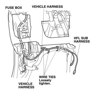
88. Route the HFL sub harness along the vehicle harness as shown. Loosely tighten it to the vehicle harness with two wire ties.
