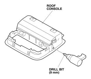
50. Measure and pierce six location on the roof console with a pushpin as shown. Drill with 3 mm drill bit on six pierced points. Widen the hole with 10 mm drill bit.
