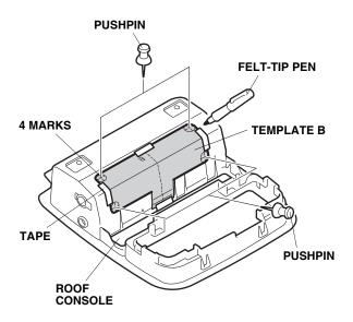
39. While wearing eye protection, drill the four marked locations to 20 mm. First drill with a 3 mm drill bit and finish with a 20 mm hole saw.
