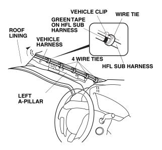
77. Route the HFL sub harness to the roof console opening.
