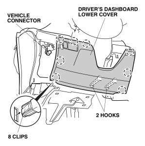
17. V6 Model only: Remove the driver's dashboard under cover (three clips and one pin).
