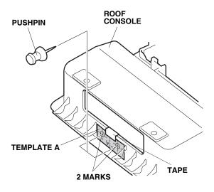
56. While wearing eye protection, drill the two marked locations to 4.5 mm. Remove any burrs.
