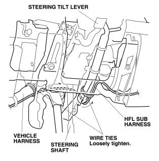
89. Route the HFL sub harness as shown. Loosely tighten it to the vehicle harness with three wire ties.
