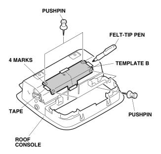
59. While wearing eye protection, drill the four marked locations to 20 mm. First drill with a 3 mm drill bit and finish with a 20 mm hole saw.
