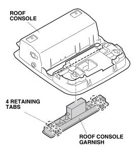
32. Remove the console light from the roof console (four retaining tabs).
