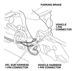
92. Secure the HFL sub harness connection part with a wire tie.
