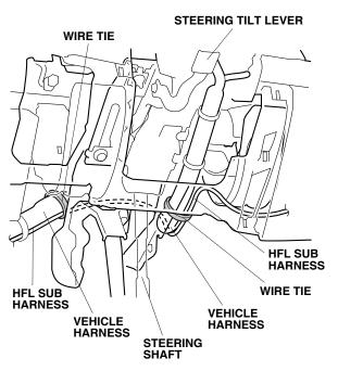
96. Tighten the three wire ties you attached in step 87.
