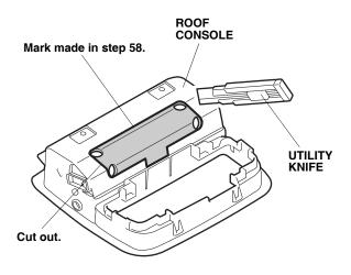
62. Using isopropyl alcohol on a shop towel, clean the areas where the double-sided tape A will attach. Remove the adhesive backing from double-sided tape A and attach the double-sided tape A at the measurements shown.
