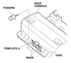
36. While wearing eye protection, drill the two marked locations to 4.5 mm. Remove any burrs.
