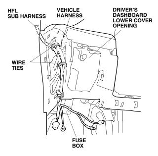
82. Plug the HFL sub harness12-pin connector into the fuse box.
