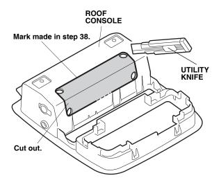
42. Using isopropyl alcohol on a shop towel, clean the areas where the double-sided tape A will attach. Remove the adhesive backing from double-sided tape A and attach the double-sided tape A at the measurements shown.
