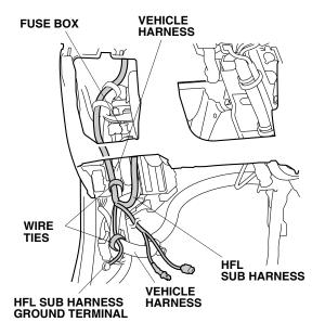
85. Install the 2 A fuse to the fuse box at the location shown.
