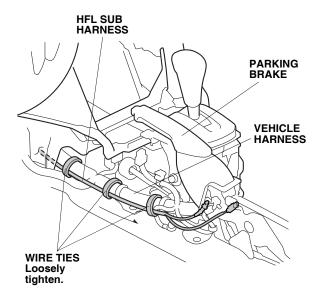
91. Disconnect the vehicle harness 1-pin connector and connect the HFL sub harness 1-pin connector in between.
