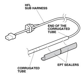
73. Wrap a wire to the sub harness as shown. Route a wire and pull the sub harness through the driver's dash board under cover opening to the left A-pillar opening.
