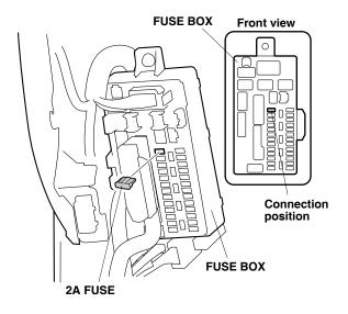
86. Attach the 2 A fuse label to the kick panel at the location shown.
