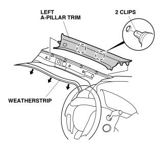
15. Remove and discard the clip from the left A-pillar trim, and install a new clip (supplied) on the left A-pillar trim.
