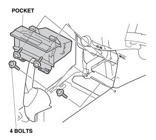
26. Remove the CD changer (two bolts, two clips, and disconnect the vehicle connector). Go to step 28.
