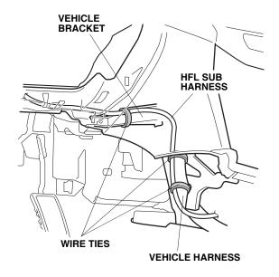
95. Tighten the three wire ties you attached in step 88.
