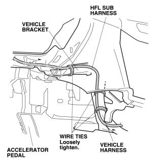
90. Route the HFL sub harness along the vehicle harness. Loosely tighten it to the vehicle harness with three wire ties.
