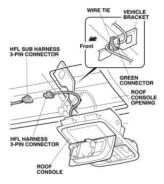
79. Using isopropyl alcohol on a shop towel, clean the areas where the EPT sealers will attach. Under the roof liner, secure the HFL sub harness to the roof panel with four EPT sealers.
