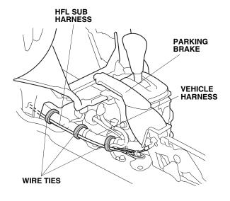
94. Tighten three wire ties from step 89.
