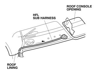
78. With an assistant holding the roof console near the roof console opening, plug the HFL harness 3-pin connector into the HFL sub harness 3-pin connector, and secure the connector to the vehicle bracket with one wire tie.
