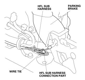
93. Tighten three wire ties from step 90.
