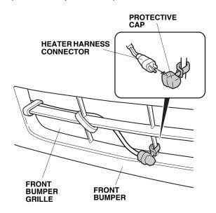
23. Route the heater harness inside the bumper, and secure it with three black wire ties.
