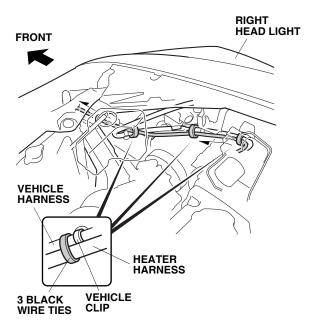
20. Route the heater harness as shown, and secure the wire tie with clip (points G) to the vehicle frame.
