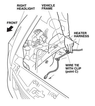
15. Route the heater harness as shown, and secure the wire tie with clip (point D) to the vehicle frame.
