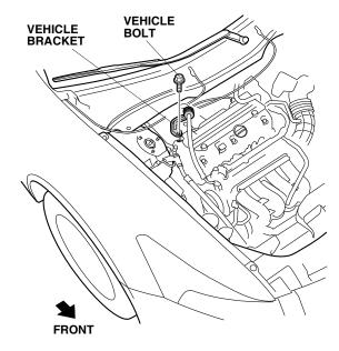
7. Disconnect the vehicle connector from the ABS or VSA modulator, and release the harness clip from the vehicle bracket.
