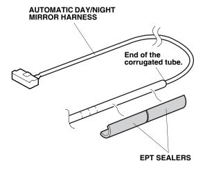
23. Attach a piece of wire to the automatic day/night mirror harness connector, and wrap electrical tape around the wire and the automatic day/night mirror harness. Route the harness to the left A-pillar trim opening.
