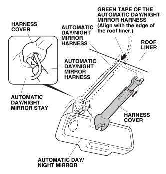
28. Slide the harness cover under the roof liner.
