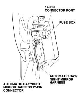
If another accessory connector is plugged into the 12-pin connector, remove the dummy connector from the other 12-pin connector harness and connect the 12-pin connector into the other accessory harness.
