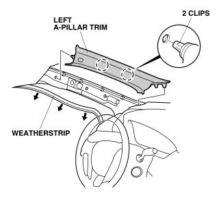
13. Remove and discard the clip from the left A-pillar trim, and install a new clip (supplied) to the trim.
