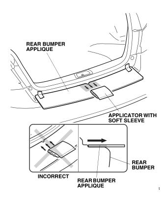
11. Starting from the center and working outward, use the applicator with soft sleeve to smooth the rear bumper applique. Repeat for right side. Stroke in one direction only.
