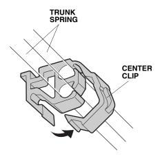
17. With an assistant holding the trunk lid open, remove the old right trunk spring from the trunk hinge arms using the trunk spring tool. Wear gloves to protect your hands, and pull the trunk spring tool slowly and carefully toward you. Do not remove the old left trunk spring.
