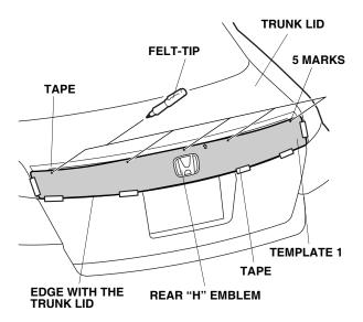
4. Position template 2 (portion A) with the center mark on the tape. Using a felt-tip pen, mark the tape at the notch as shown.
