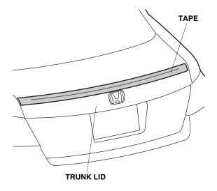
3. Close the trunk lid. Align template 1 with the rear "H" emblem and edge with the trunk lid. Tape template 1 to the trunk lid. Using a felt-tip pen, mark on the tape as shown. Remove template 1.
