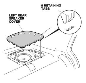
10. Remove the left rear speaker (one bolt and disconnect the vehicle connector).
