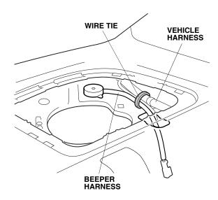
24. Plug the beeper 2-pin connector into the back-up sensor harness 2-pin connector.
