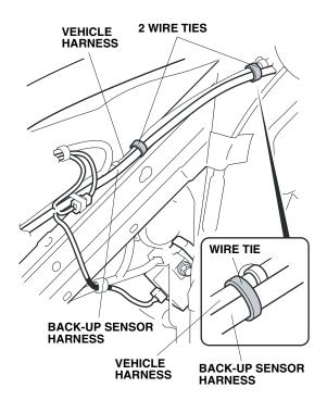
18. Secure the back-up sensor harness clip to the hole in the vehicle panel.
