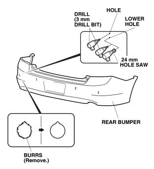
Using a 24 mm hole saw, enlarge the upper outboard hole on the left side of the bumper. Remove all burrs.
