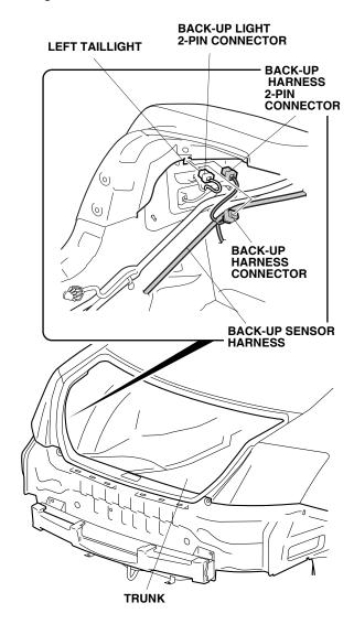
15. At the left taillight, secure the back-up sensor harness to the vehicle harness with one wire tie.
