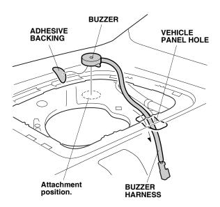
22. Remove the adhesive backing from the beeper, and attach it to the opening in the left rear speaker at the location shown. Route the beeper harness through the hole in the rear shelf.
