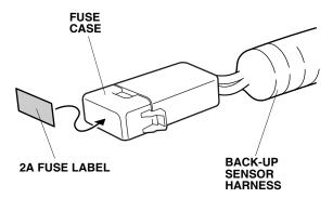
14. Disconnect the back-up light 2-pin connector from the left taillight, and plug it into the back-up sensor harness 2-pin connector. Plug the remaining back-up sensor harness 2-pin connector into the left taillight.
