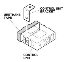
12. Install the control unit to the vehicle panel:
