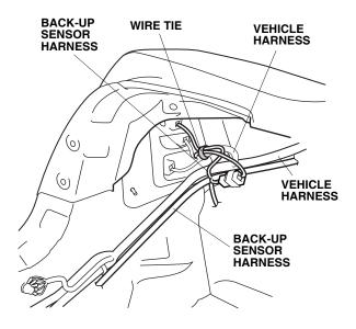
16. Plug the back-up sensor harness 14-pin connector into the control unit, and route the harness forward along the vehicle harness. Secure the back-up sensor harness to the vehicle harness at the green tape.
