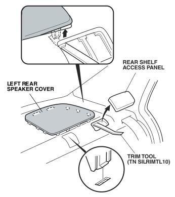
9. Remove the left rear speaker cover (nine retaining tabs).
