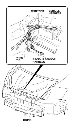
28. Install one wire tie with clip to the holder with the fuse case, and attach the wire tie to the vehicle harness.
