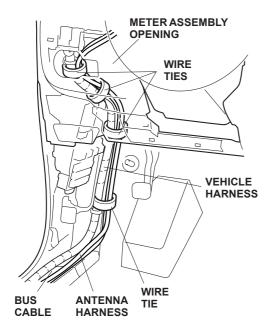
36. Route the bus cable as shown. Secure the bus cable and antenna harness to the vehicle harness using two wire ties as shown.
