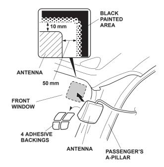
16. Route the antenna harness down the passenger's A-pillar along the vehicle harness, secure the antenna harness to the vehicle harness with three wire ties in areas shown.
