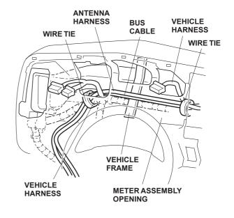
37. Align the end of the bus cable connector with the end of the vehicle 20-pin connector and secure the bus cable to the vehicle harness using a wire tie.
