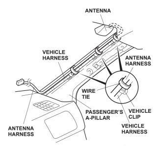
17. Using a felt-tip pen, mark the antenna harness at the point where the harness touches the dashboard.
