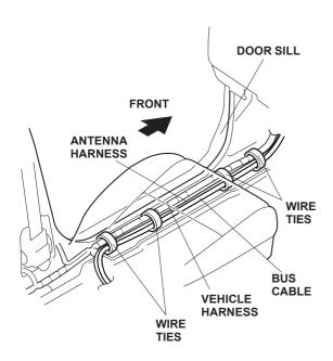
35. Route the bus cable and antenna harness as shown and secure it to the vehicle harness using four wire ties.
