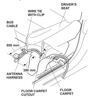
27. Bind the antenna harness and bus cable together in the position shown using a wire tie with clip.
