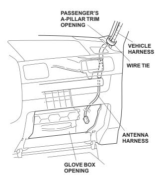
20. Inside the glove box opening, route the antenna harness along the vehicle harness and towards the driver's side of the vehicle. Secure the antenna harness to the vehicle harness with three wire ties in the areas shown.
