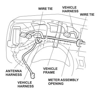
23. Route the antenna harness along the vehicle harness and temporarily secure it to the vehicle harness using four wire ties.
