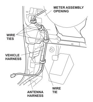
24. Route the antenna harness as shown and temporarily secure it to the vehicle harness using four wire ties.
