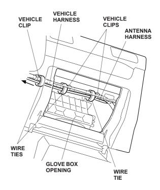
21. Route the antenna harness past the audio unit opening, and secure the antenna harness to the vehicle harness with one wire tie.
