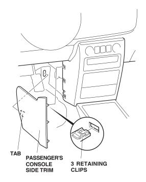
4. Remove the passenger's console side trim (two retaining clips and one tab).
