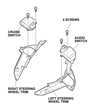
11. Install the CRUISE and AUDIO switches to the new left steering wheel trim and new right steering wheel trim with the four screws (reuse). Go to step 16.
