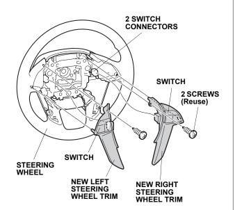
17. Install the new left steering wheel trim and new right steering wheel trim to the steering wheel with the two screws (reuse).
