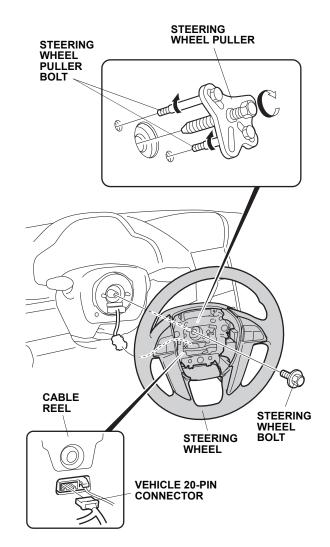
7. Remove the steering wheel bolt. Unplug the vehicle 20-pin connector from the cable reel. Using a steering wheel puller, remove the steering wheel. Do not thread the steering wheel puller bolts in more than 10 mm.
