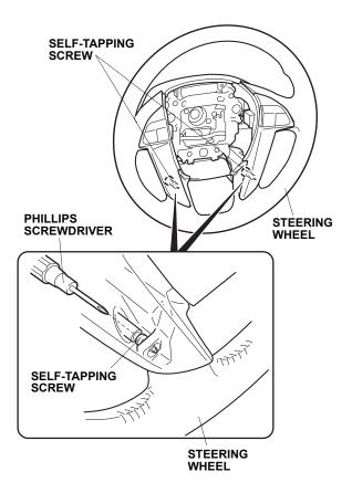
9. Remove the four self-tapping screws that fasten the left steering wheel trim and right steering wheel trim from the steering wheel and unplug the two switch connectors. Remove the steering wheel trim from the steering wheel.
