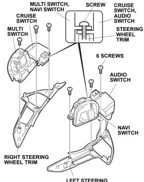
LEFT STEERING WHEEL TRIM 15. Install the CRUISE, AUDIO, MULTI and NAVI switches to the new left steering wheel trim and new right steering wheel trim with the six screws (reuse).
