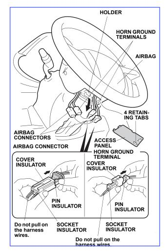
4. Remove the horn ground terminals and the airbag connectors from the holder. Unplug the horn ground terminals and the airbag connectors. While holding the pin insulator, pull out on the cover insulator. Do not pull on the socket insulator and harness wires. 5. Remove and discard the two torx bolts that secure the airbag, and remove the airbag. Carefully set the airbag in a secure location with the pad facing up. Do not drop or bump the airbag against anything.
