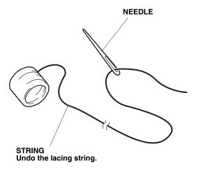
5. Starting in the back of the left spoke, lace the string through the holes of the steering wheel cover from the inside. Leave approx. 100 mm (3.93 in.) of string at the end. This will be used to tie the string at the end.
