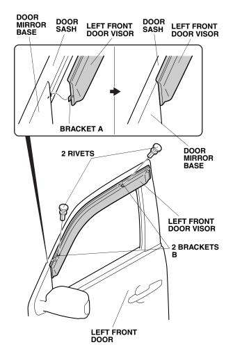
6. Align the holes on two brackets B to the holes on the left front door visor and secure it with two rivets.
