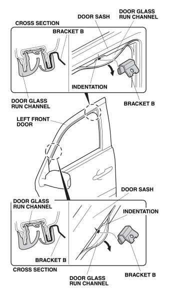
2. Peel the door glass run channel and install two brackets B to the left front door as shown. Make sure that the brackets are installed in the correct position. Check that the brackets and the door glass run channel is installed on the door sash properly. 3. Peel back approximately 1-1/2 to 2 inches of adhesive backing from each adhesive tape, and tape the ends to the front surface of the left front door visor with a masking tape.
