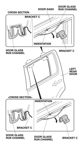
11. Peel the door glass run channel and install two brackets C to the left rear door as shown. Make sure that the brackets are installed in the correct position. Check that the brackets and the door glass run channel is installed on the door sash properly. 12. Peel back approximately 1-1/2 to 2 inches of adhesive backing from each adhesive tape, and tape the ends to the front surface of the left rear door visor with a masking tape.
