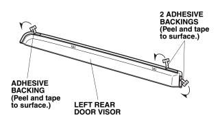
13. Using the isopropyl alcohol on a shop towel, clean the door sash where the left rear door visor will attach.
