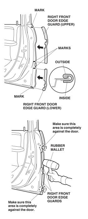
7. Repeat steps 3 thru 6 to install the left front door edge guards.
