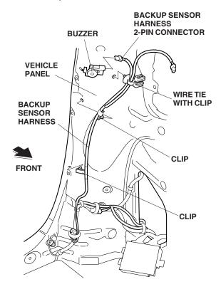
26. Install a wire tie with clip to the backup sensor harness, and secure the clip to the vehicle panel.
