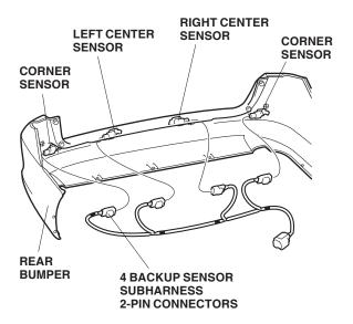
45. Secure the backup sensor subharness connector at the green tape with four wire ties.
