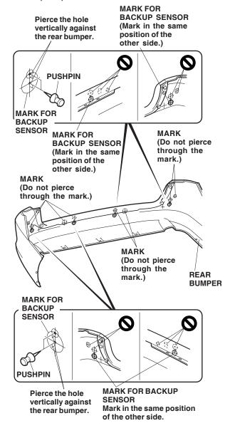
38. While wearing eye protection, drill 3 mm holes at the four pierced marks on the corner of the rear bumper from the outside. Widen the two lower holes with a 24 mm holesaw as shown. Remove any burrs.
