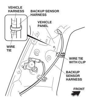
30. Secure the backup sensor 8-pin connector to the vehicle panel.
