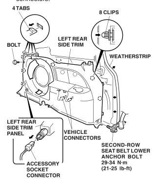
12. Remove the left rear pillar trim (one cover, one bolt, one clip, and two tabs).
