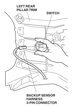
35. For the left rear pillar trim, insert the clip matching the upper tab and install the trim.
