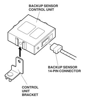
23. Attach the backup sensor control unit to the vehicle panel, and secure the control unit bracket with a 6 mm flange nut.
