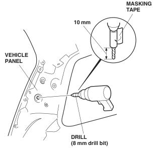
15. Install the blind nut into the 8 mm hole you drilled in step 14. Attach the buzzer to the vehicle panel using the 4 x 14 mm washer-screw. If equipped with a vehicle harness, disengage the vehicle clip from the vehicle panel. Remove the tape and the vehicle clip. Attach the harness clip to the vehicle harness with the tape as shown. Secure the buzzer to the vehicle clip before installing it to the vehicle panel.
