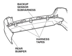
47. Bring the rear bumper to the vehicle, and connect the backup sensor subharness 8-pin connector to the backup sensor harness 8-pin connector.
