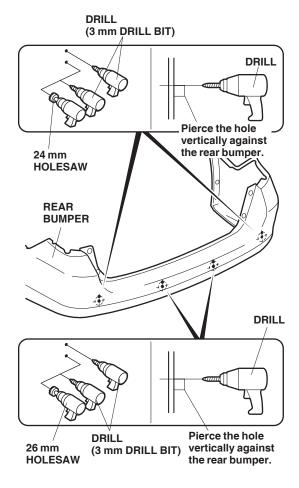
39. While wearing eye protection, drill 3 mm holes at the four pierced marks on the center of the rear bumper from the outside. Widen the two lower holes with a 26 mm holesaw as shown. Remove any burrs.
