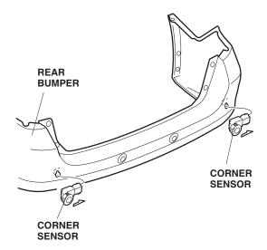
43. From the inside of the rear bumper, insert the two corner sensor clips to the two corner sensors.
