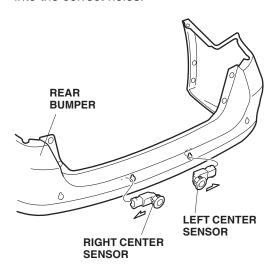
41. From the inside of the rear bumper, insert the right center sensor clip (black) and left center sensor clip (white) to the right center sensor and left center sensor.
