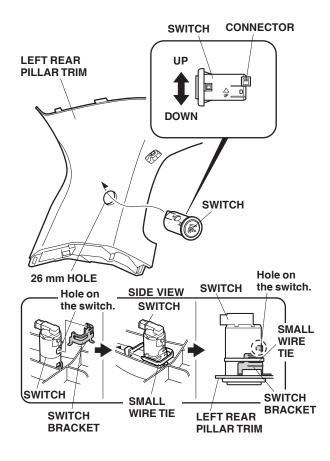
33. Secure the switch bracket to the switch with a small wire tie.
