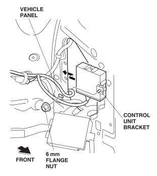
24. Secure the backup sensor to the vehicle harness with one wire tie.
