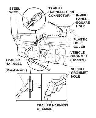
8. Remove the steel wire from the trailer harness 4-pin connector.
