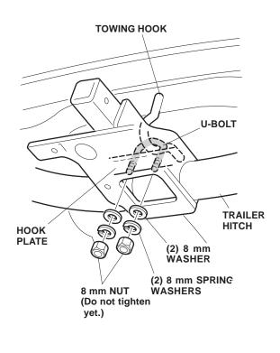
27. Torque all bolts and nuts to their specified torques in the order shown.
