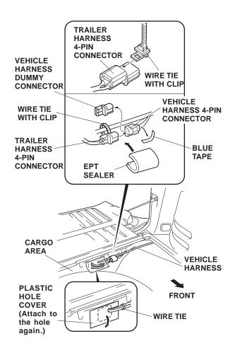
10. Secure the trailer harness to the vehicle harness with one wire tie as shown. Route the trailer harness through the square hole in the inner panel and attach the plastic hole cover that you turned up before to the hole again. 11. Route the trailer harness down through the clearance between the rear bumper beam and body panel. Reinstall the rear bumper.
