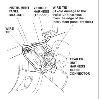
21. Secure the 10-pin connector connected in step 17 with a wire tie to the vehicle harness.
