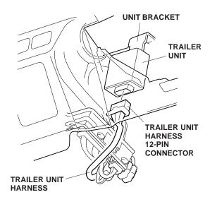
20. Secure the trailer unit harness with a wire tie to the instrument panel bracket.
