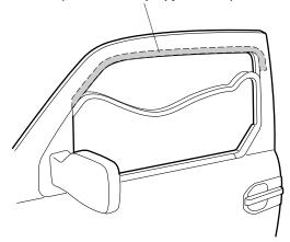
Attach a strip of the masking tape to the ends of the adhesive backings, and remove 5 to 8 cm (2 to 3 in.) from the ends. Fold back the ends and tape the ends to the front of the door visor. Note the direction of the adhesive backings.
