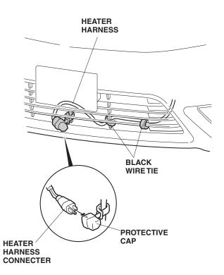
24. Attach the protective cap to the grille, and plug the heater harness connector into the protective cap.
