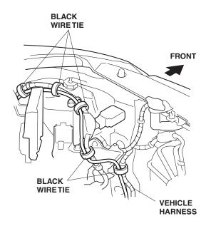
23. Route the heater harness on the inside of the bumper opening and secure it to the grille with two black wire ties.
