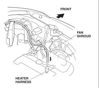
21. Secure the wire tie with clip (installed on the heater harness in step 11) to the vehicle frame, and route the heater harness to the front bumper opening.
