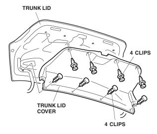
On the inside of the trunk lid, locate the identification marks on the trunk lid. Lightly centerpunch the mark. Repeat on the right side of the trunk lid.
